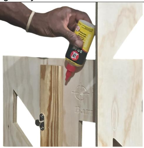
PTSB's are made largely of wood and plywood and therefore are subjected to contraction and expansion depending on the environment where they are stored or used. Sometimes excessive expansion may reduce the ease with which the detachable portion slides up/down. Adding lubricant in the sliding tract may promote smoother sliding during height adjustment.
