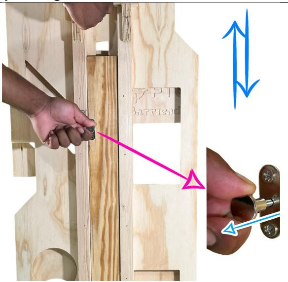
Adjust the height of the barricade as needed by pulling the knob of the dowel lock. Pull the knob while raising or lowering the detachable portion then simultaneously releasing the knob so that it selects the next adjustment slot milled into barrier.
